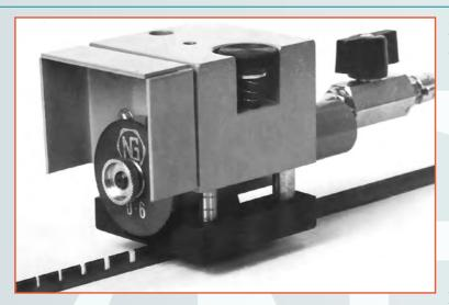
The grinding head moves smoothly on linear ball bushings along precision ground, hardened steel shafts.
