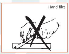
These methods of nicking produce inferior quality "nicks" with low tensile strength at the risk of bending and deforming the cutting rule.
